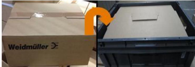
**Figure 10:** Illustration of the use of modular cardboard carton inserts (left) in euro norm containers (right)
